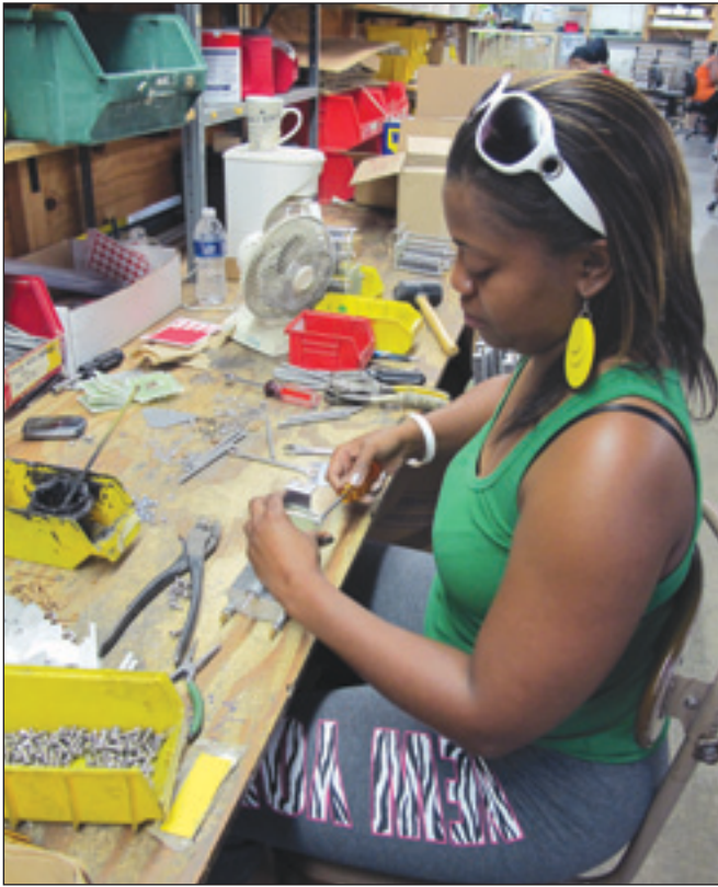
With a variety of parts within reach, Shonda Warren assembles an air variable capacitor for an antenna tuner.
