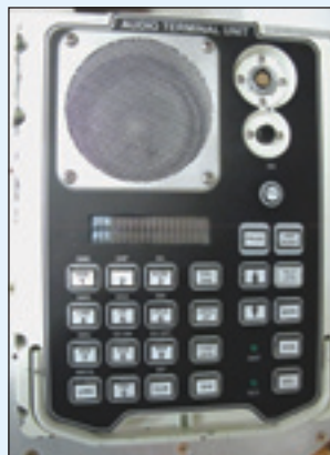
A communications panel in the Columbus module of the ISS. These are used for both internal communications within the spacecraft and for radio communications with the ground controllers. These are familiar looking controls to radio operators: XMIT Mode, VOX, VOL and PTT. A ham would feel right at home.
