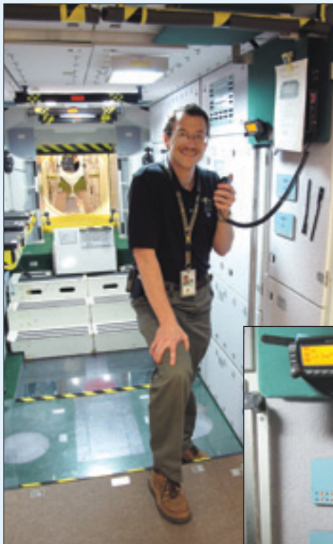
Kenneth Ransom, N5VHO, ISS Ham Radio Project Coordinator, demonstrates the Kenwood dual-band TM-D700 144/440 MHz Amateur Radio transceiver mounted against the wall in the Russian Service Module mockup, the same area that it is located in the ISS. NASA engineers will also be installing an Ericsson Radio system in the Columbus Module (ESA) training mockups at JSC similar to the actual ISS installation. There is no chair for the operator. In micro gravity, the astronaut/radio operator floats next to the radio.
